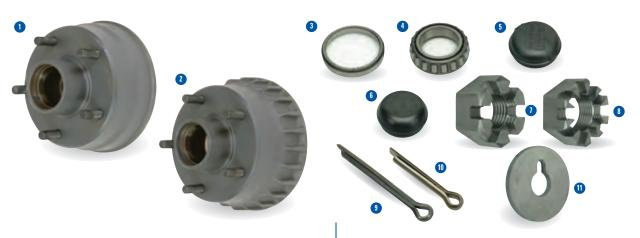
KS0755L Brake drum. From 20th June 1988 for 6.00x9 wheels. Complete with 2 off bearings P0001 /P0002, oil seal P0004, bearing retaining washer C14679, axle end nutF1099S, grease cap C72253, 5 off wheel stud F1804, 5 off wheel nut F1813, spirol pin F1909S and split pin F1508.
